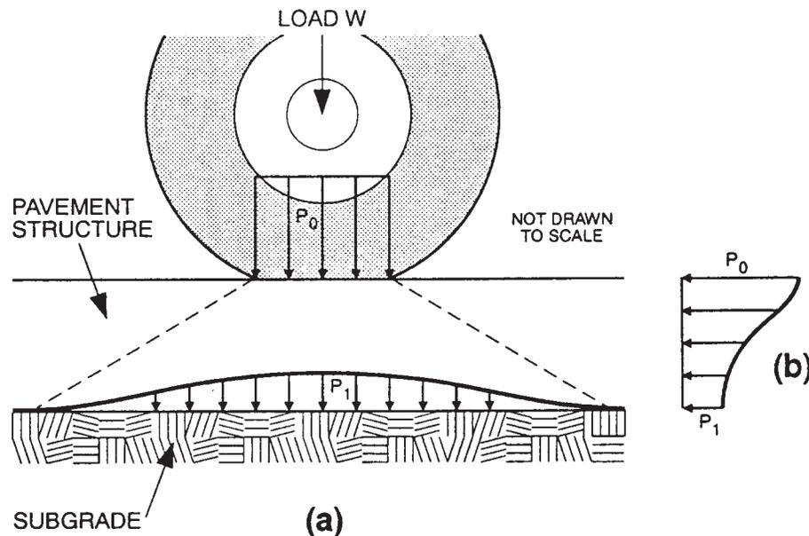
**Figure 3-1.** Spread of wheel-load through pavement structure.
