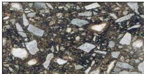
60% Crushed, Type "A" Aggregate
