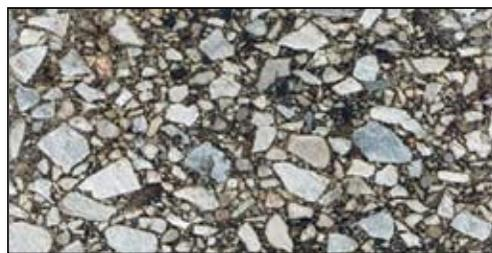
75% Crushed, Type "A" Aggregate
